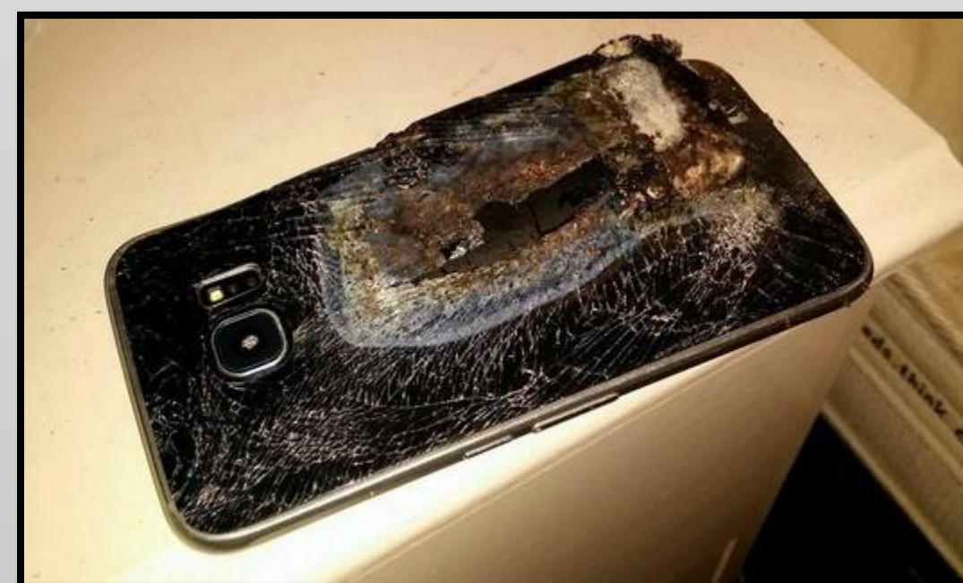
Figure 4: SAMSUNG Li-ion battery explosion Li-ion battery ignition can cause major damage to both property and those in the vicinity - (Image: SWNS) http://www.mirror.co.uk/news/uk-news/mums-samsung-phone-explodes-bursts-7575275
