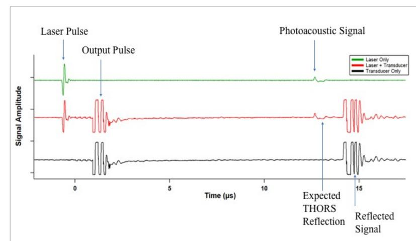
Fig 3. Ultrasound Reflection in no dye tissue phantom at 532 nm
