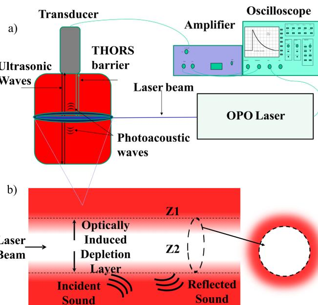
Fig 1. a) Experimental setup using ultrasound
