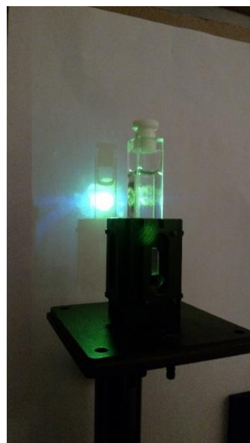
Fig. 1: A sample of cyclohexane subjected to 213nm light in an effort to generate a Raman spectrum.
